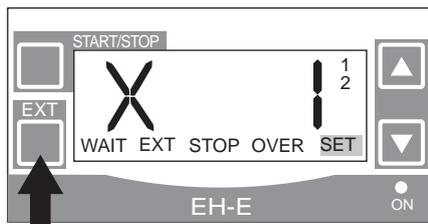
If you push EXT key, the display changes to X 1 (Multiplying operation). Every time EXT key is pushed, X 1 and / 1 are switched over.
