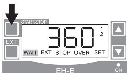
(6) Push START/STOP key to confirm the digital mode and move to wait mode.
