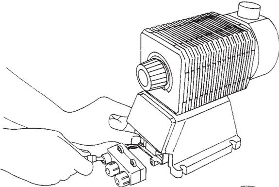
6) Mount terminal box on case in the manner the connection label comes upside and fix it with attached four screws. Tightening torque is 0.5 N•m.
