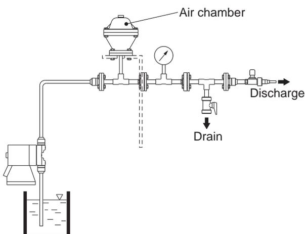
6. Install of accumulator or air chamber
