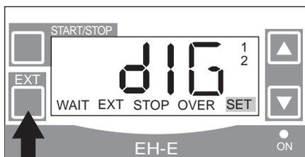
(5) Push EXT key to confirm ON, OFF of pulse memory and return to EXT operation mode.
