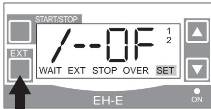
(3) Move to pulse memory (The function to put in memory the pulses (max. 255 pulses) which come while the pump does the multiply operation.)
