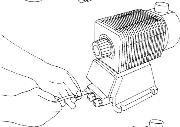
7) Adjust the tension of cord inside terminal box and insert cord gasket into terminal box.
