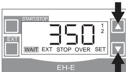
When the spm value is changed, the value is not put in memory unless you push START/STOP key or EXT key, or until three or more seconds have passed.
