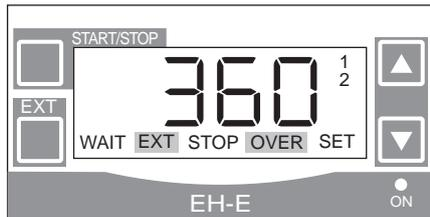
When analog input being set, if the same value (current or stroke rate) is put for SET point 1 and 2, ERR 1 is displayed for three seconds and then returns to set display.
