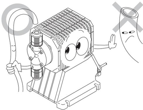
4. Use the tube corresponding to the pump suction and discharge port sizes. Securely connect the tube so that liquid can not leak or air can not be sucked in.
