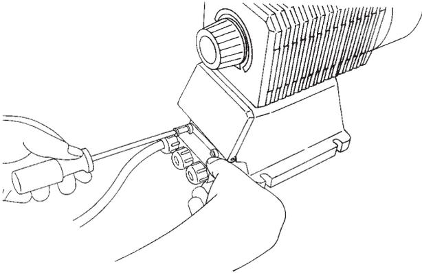
1) Remove four screws with screw driver to take off terminal box.
