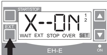
If X -- ON or X -- OF is displayed, push EXT key and the display changes to / -- ON or / -- OF. (Every time you push EXT key, / -- OF or / -- ON, X -- ON or X -- OF switches.) When the pump is shipped from the factory, it is set at X -- OF.
