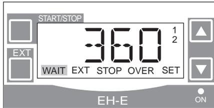
(2) Stroke rate can be changed by pushing ▲ or ▼ key at wait mode or during operation. Push ▲ key to increase stroke rate and ▼ key to decrease. If you push the key in a short time, the spm figures changes slowly by one spm and if you continue to push over three seconds, they change quickly. The pump is shipped set at 360 spm.
