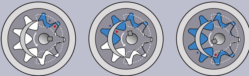
A pinion (drive gear) coupled with a shaft supported by two bearings meshes with an internal gear (driven gear) whose periphery is supported by a strong bearing. Liquid is transferred by a change in the capacity of this meshed portion. In the suction process, the gears are disengaged and a space defined by the two gears and the casing expands. The
