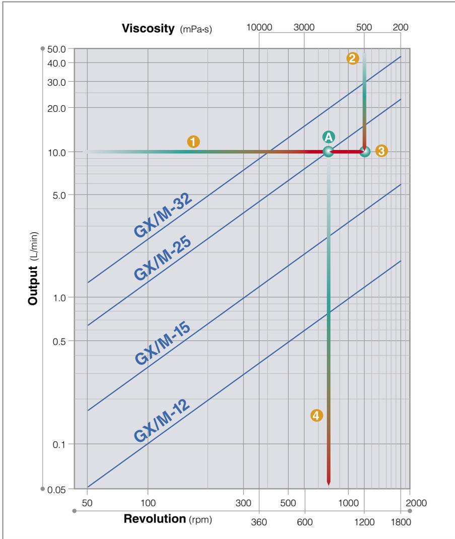
The chart on the left shows output at a discharge pressure of 0MPa. The output changes in proportion to rpm, but rpm should be reduced when pumping viscous liquid. Knowing required output and viscosity, the proper pump/motor rpm can be selected as in the following example.
