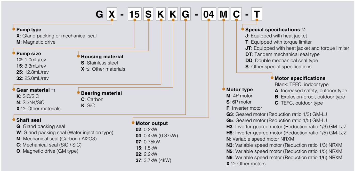
\*1. Pinion/Internal gear \*2. Special specifications
