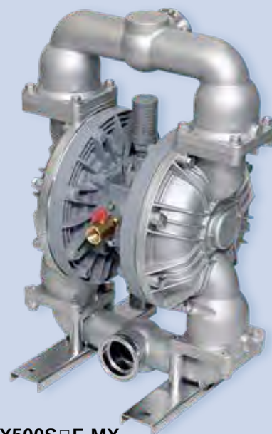
TC-X500S □ F-MX FDA Type Electro Polished SUS Pump. 2½" Sanitary Flange Connections. 520 L/min Max Flow Rate. (PTFE Diaphragms) 8mm Max Solids Size.
